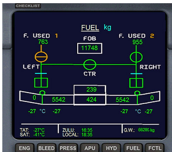
Picture 40 – CROSSFEED open with the 2 fuel pumps
