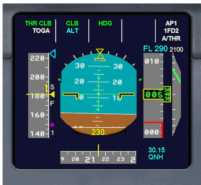
Picture 63- VNAV has engaged the autopilot in HDG mode
