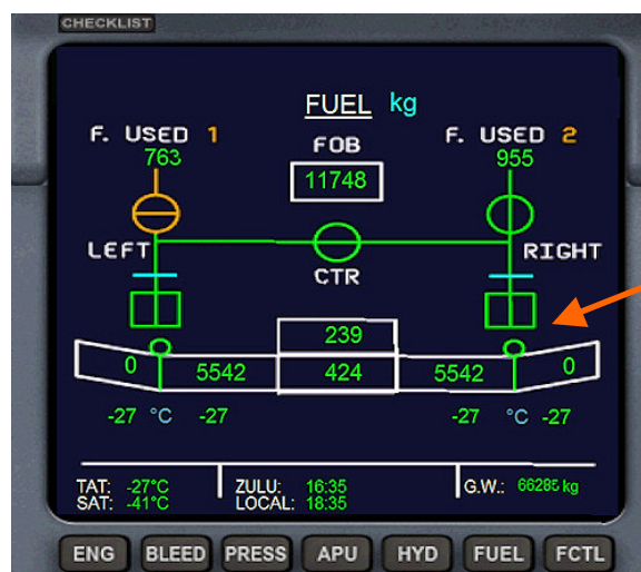
Picture 39 – CROSSFEED opened, and all pumps run : all tanks are open
