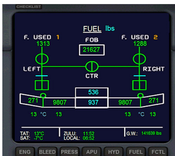
Picture 27 – Secondary ECAM FUEL page
