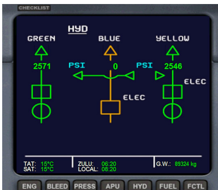
Picture 26 – Secondary ECAM - HYD page
