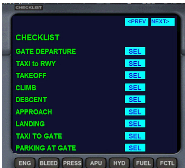
Picture 20 – secondary ECAM Checklist main menu Page
