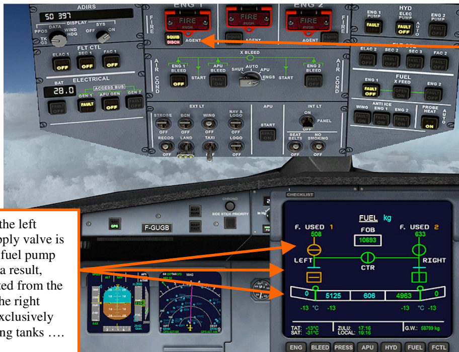
Picture 76 – Fire is out. We'll have to manage the fuel system to prevent the plane imbalance .... Please, note that this screenshots comes from the Airbus A319, which have just one center tank...
